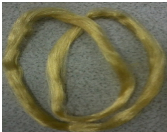
Fig. 2. Photograph of the chitosan/cellulose composite fiber prepared by dry-wet spinning.
